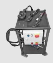
Electric hydraulic power unit (for GR 1, GRM 1 and GRT 1 hydraulic heads) with trolley and WB 6 extension arm form integrated work site enabling work with three different heads.
