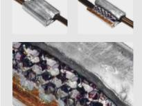
In connection made with Shark technology, teeth of the connector bite through the enamel and into the core of connected wires. Therefore made connection is electrically and mechanically reliable.
