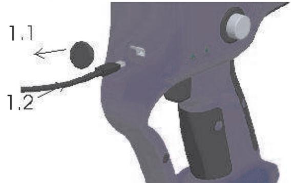
Connection of mini-USB-cable to tool
