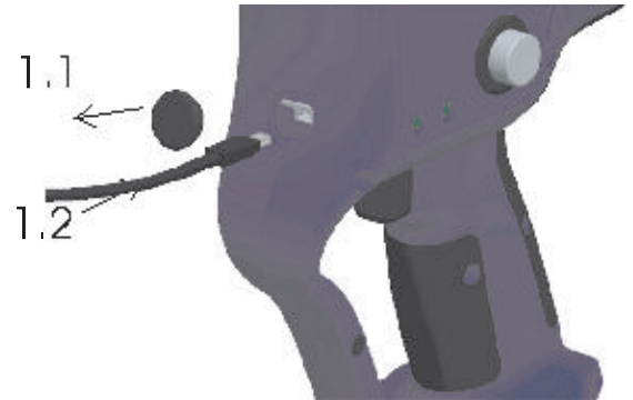
Connection of mini-USB-cable to tool
